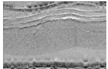
*Sidescan data from Worbarrow Bay. The main reef running across the bay is clearly visible. Close examination also reveals a small wreck (thought to be the Patricia II) and parts of the Winfrith pipeline.*
