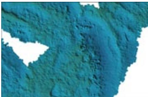
Section of multibeam data from CEFAS showing area of large boulders
